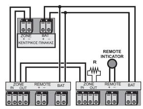
Remove the protective cover and connect the power supply and the zones to the connecting terminals.
